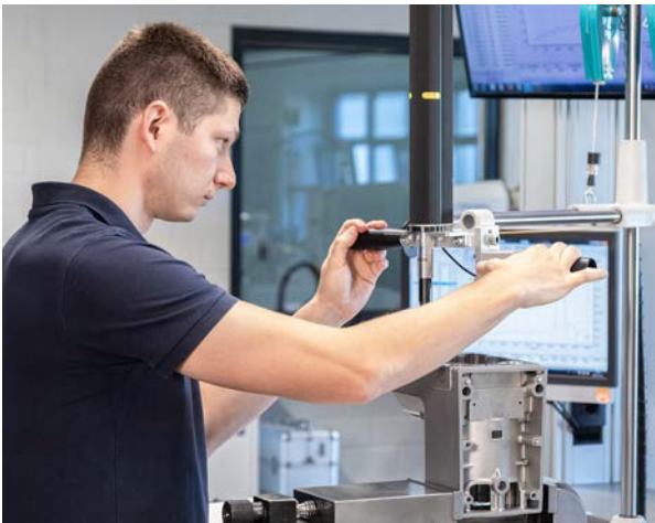
Lab expertise: qualified application engineers set the screw-in parameters for our customers' components.
