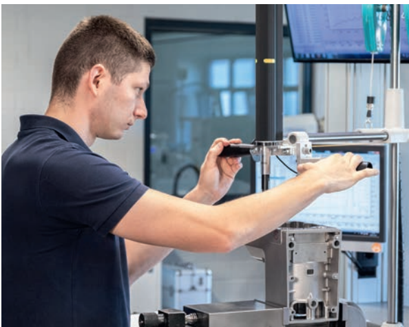
Lab expertise: qualified application engineers set the screw-in parameters for our customers' components.
